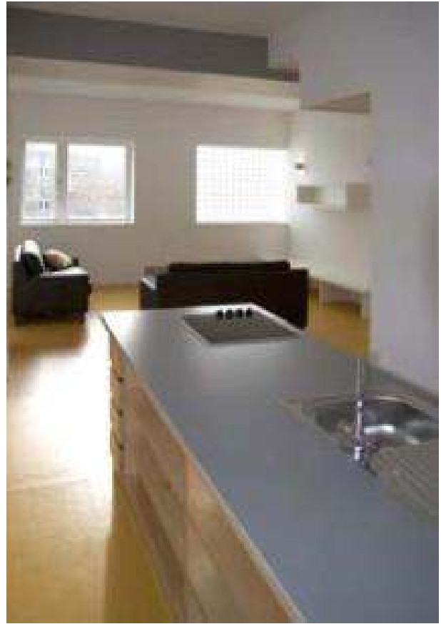
Kitchens units are bespoke birch ply doors and carcasses
