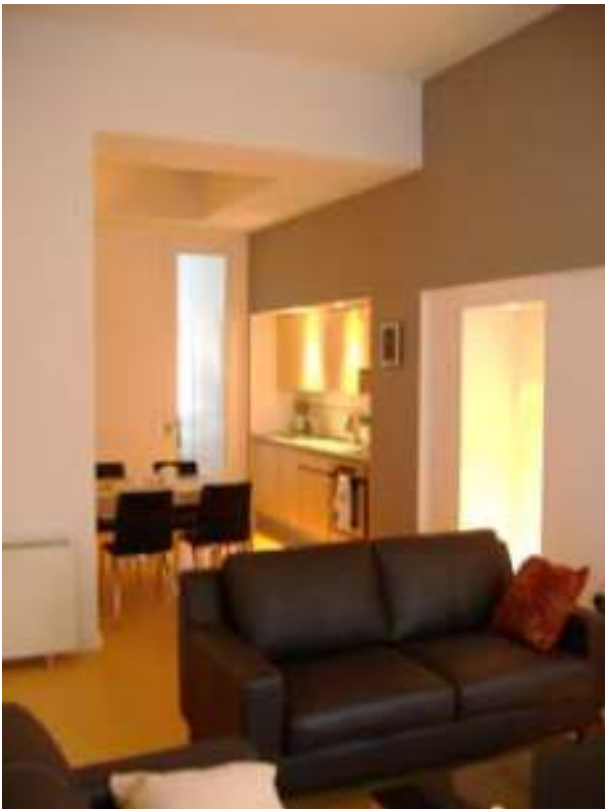
Floor finishes throughout are of rubber sheeting, on a sound impact underlay
